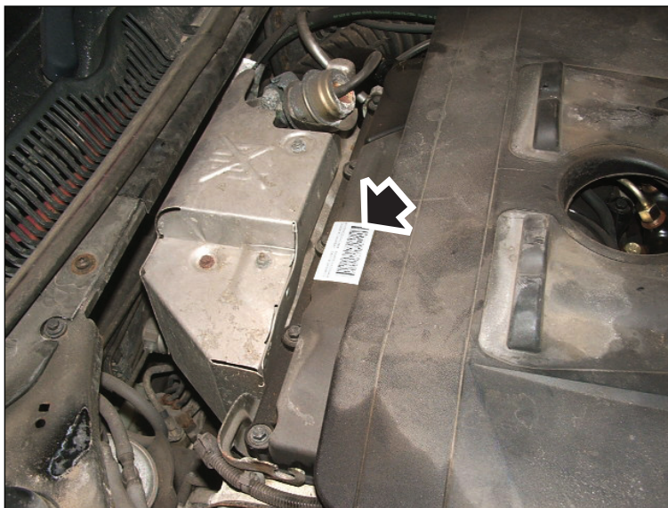
2.0 TDCi Engines: - Injector label arrowed in illustration - Side view
