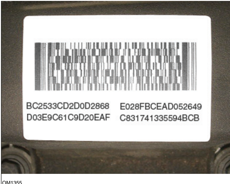
Injector label - gives four 16 digit numbers
