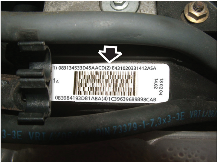
Injector label - gives four 16 digit numbers
