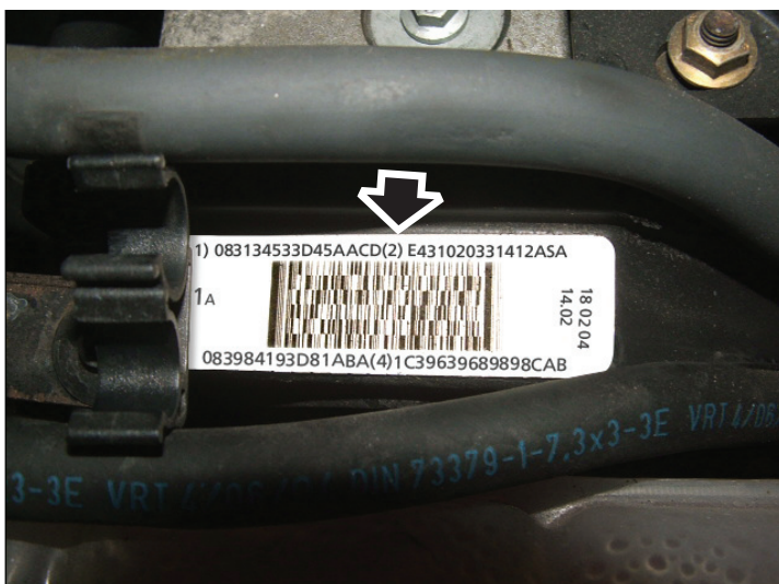
Injector label - gives four 16 digit numbers
