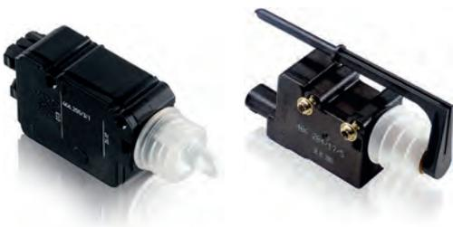
These actuators are controlled by the central locking system and/or remote control. Each actuator's motor operates a lifter that activates and deactivates the lock. Additionally, the lifter may be retained by a latch mechanism and used specifically for anti-theft protection.
